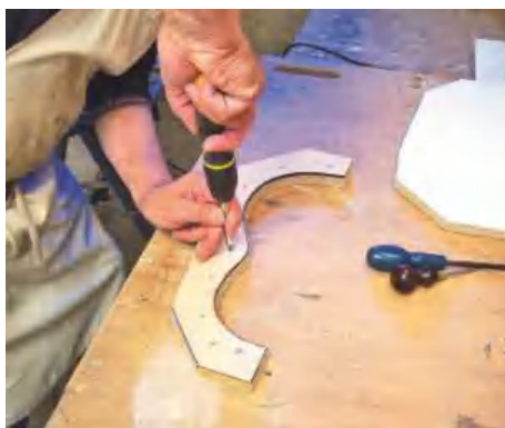
▲ Pic.5 Attaching the template onto a side piece
